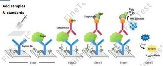
Step1: Add 100ul standard or sample to each well and incubate at 2-8°C for 16h (2-8°C overnight).
